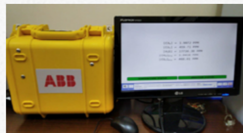
Figure 2: Microportable Greenhouse Gas Analyzer LGR-ICOS™ GLA Series
